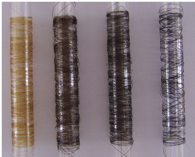
Fig. 2. Photograph of PBO and PBO–MWNT composite continuous fibers collected using spools. The MWNT composition increases from left to right, namely, 0, 0.18, 0.36, and 0.54 wt%.
